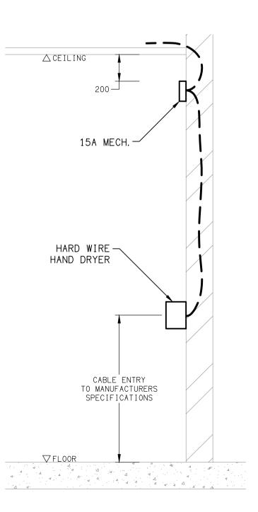
**DETAIL** HAND DRYER CONNECTION NOT TO SCALE
